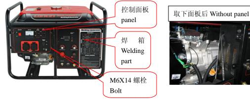
2、取焊箱: 松开焊箱安装螺栓 (左右各三颗 M8X10 螺栓, 10#套筒),取下焊箱; Release 6 pcs of bolt M8X10 by 10# sleeve to knock down welding part
